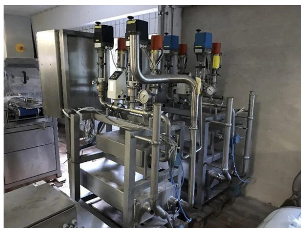
Slika 3. Standardizator (Kompomaster) (secondhand-equipment, URL)
