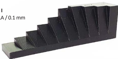
UZORAK II FDM / PLA / 0.2 mm
